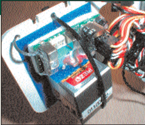
Hitec RCD's GY-130 Piezo Gyro (bottom) keeps the Lite Machines Corona 120 helicopter stable in the yaw axis.
