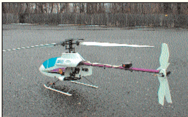
FMA's Co-Pilot is installed in this Lite Machines Corona 120 electric helicopter. In following issues, the amazing FMA Co-Pilot Flight Stabilization System will be flown as you see it here, and in a 40-class RC trainer and in a motor-glider.
