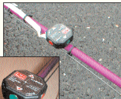
The Co-Pilot sensor mounts outside the aircraft, away from fuel spray
