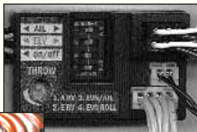
Co-Pilot's Computer mounts inside the aircraft. It connects between the pitch and roll servos and the receiver. Reversing switches are provided, as is a gain control to adjust the unit's sensitivity.
