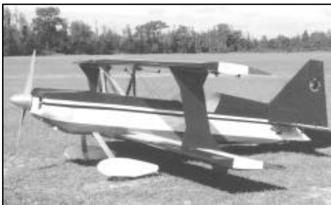
Now here is an Ultimate! Product of Bob Godfrey. 42%, DA150 engine, 40#, JR radio. An awesome aircraft. The bigger they are the more realistic they appear.
